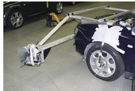
Infrared camera ready to measure rolling resistance and other tyre features
